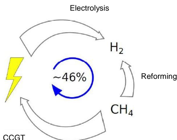
Legend: If we convert methane (CH<sub>4</sub>) into electricity by using the most efficient technology, and then extract hydrogen from it, through electrolysis, we will have transformed methane into hydrogen, which is what the current “grey” hydrogen process already does by reforming, and with a consumption of methane that is at least twice as low!
